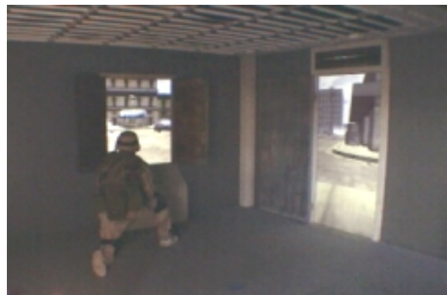
Figure 5. User viewing OGRE scene presented on two wall sized displays with physical door and window props. An unmanned aerial vehicle (UAV) appears in the window.
